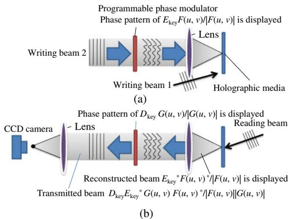
Fig. 4. (Color online) Optical setup of the optical correlator based on phase-only correlation using holographic memory and phase modulator. (a) Recording process of reference data. (b) Image-matching process.
